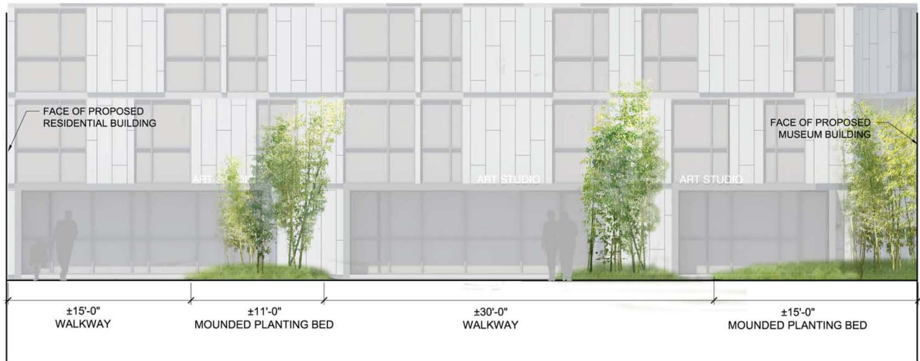
COURTYARD ELEVATION B-B
